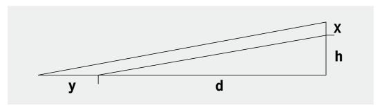
Figure 1. A relatively small increase (x) in the height (h) of the harpoon as a wave lifts the bow of the ship, results in a large change in projection (y) of a harpoon aimed just before the wave at a whale at a distance (d) from the whaling ship, which would have to be compensated during the wave motion in order to try to maintain the aim (for further explanation see the text).
